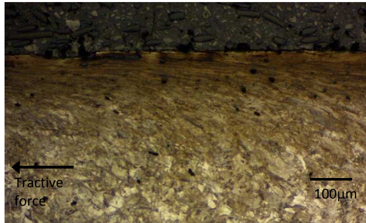
Figure 22: Image of the running surface of the premium rail disc in cross section displaying ratchetting behaviour
