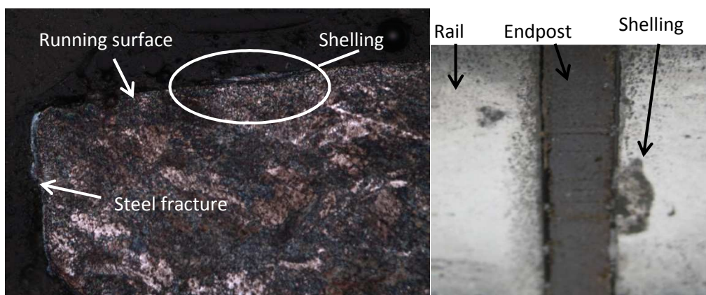
Figure 10: Comparison of shelling in a) the twin disc test and b) in the field [4]
