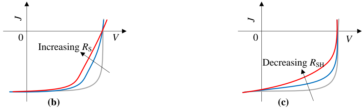
Figure 2.11: Effect of (a) increasing R_S and (b) decreasing R_{SH} , on J - V characteristics of the solar cell (Adapted from Nelson, 2003).
