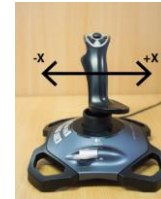
Figure 4 The joystick control interface and the axis uses to control the pendulum angle.
