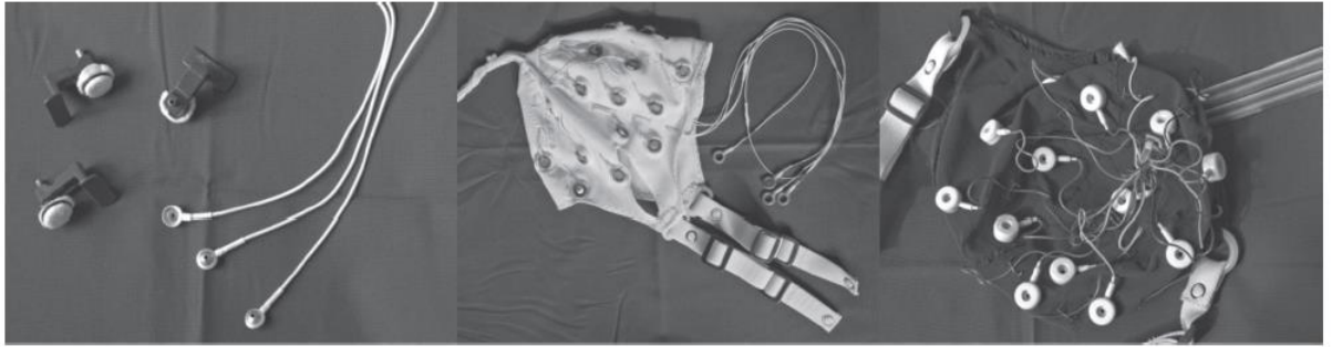
Figure 2.19 The electrodes and caps for EEG data acquisition [166].
