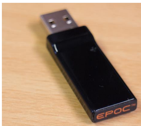
Figure 2.24 USB dongle for wireless data acquisition with the Emotiv EPOC headset.
