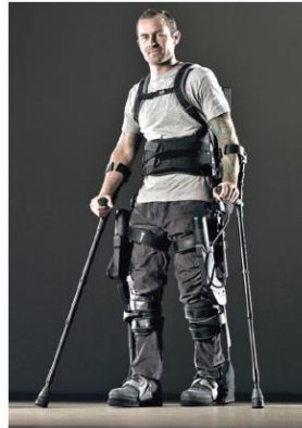
Figure 1.3 A fully lower limbs exoskeleton support system [3], [4].
