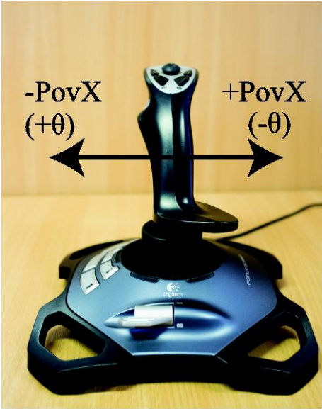
Figure 4.9 The joystick and the axis mapping to the pendulum angle.
