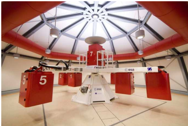
Fig. 4. The Large Diameter Centrifuge (LDC). (courtesy ESA)
