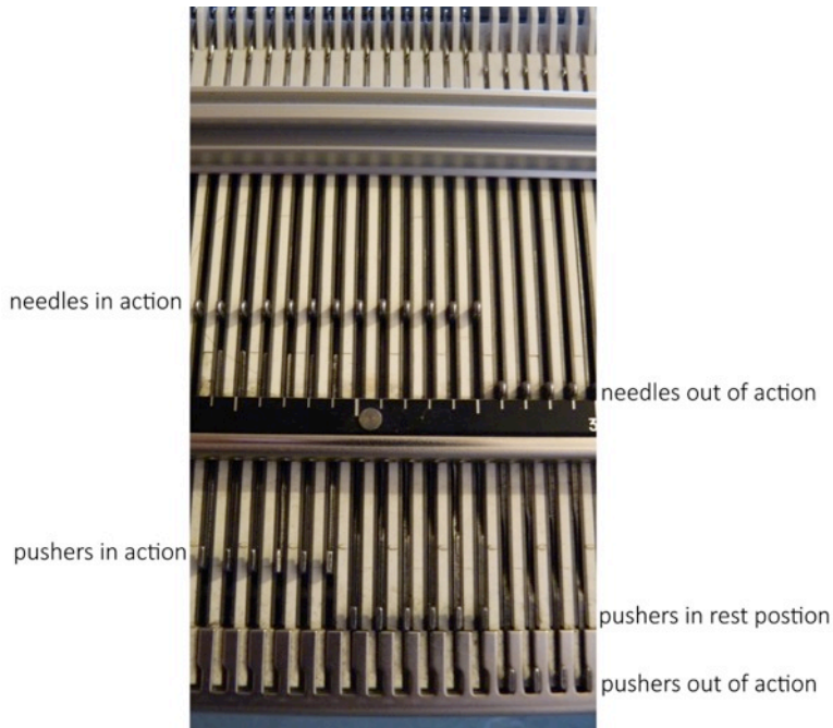
Figure A4.6. Passap, needle and pusher positions.
