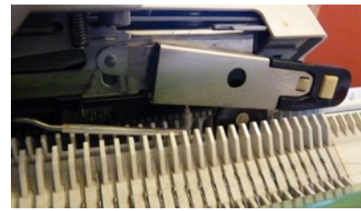
Figure A4.12. Action of a single bed, Passap stripper.
