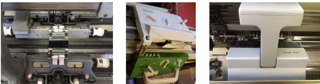
Figure A4.2. Cam box (left to right) Dubied, Passap and Shima Seiki SES double system. (J. Taylor)
