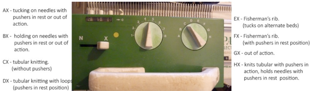
Figure A4.8. Passap pattern selector and pattern options. (J. Taylor)
