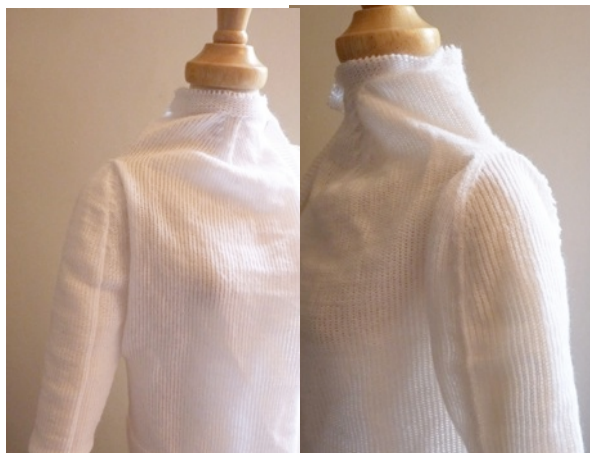
Figure 8.13. Pleat sleeve with fashioned sleeve head and parachute shaping across shoulders.
