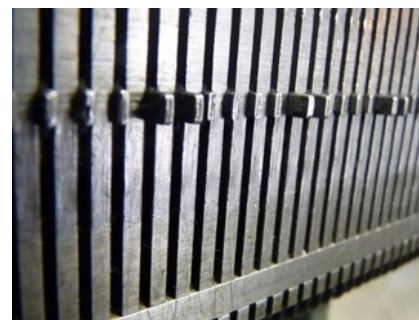
Figure A4.7. High and low butts on a Dubied hand-flat knitting machine.
