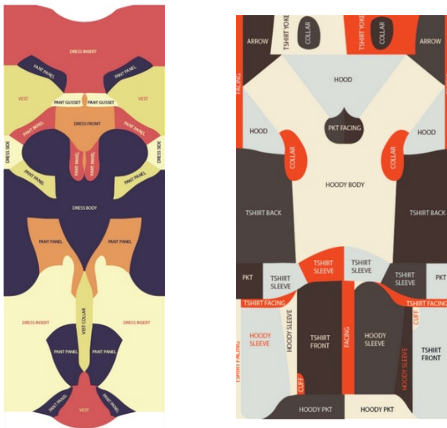
Figure 6.5. Zero-waste pattern layouts by Holly McQuillan. ( http://hollymcquillan.com/images/#ip-carousel-606 ) (Permission to reproduce this image was granted by H. McQuillan)
