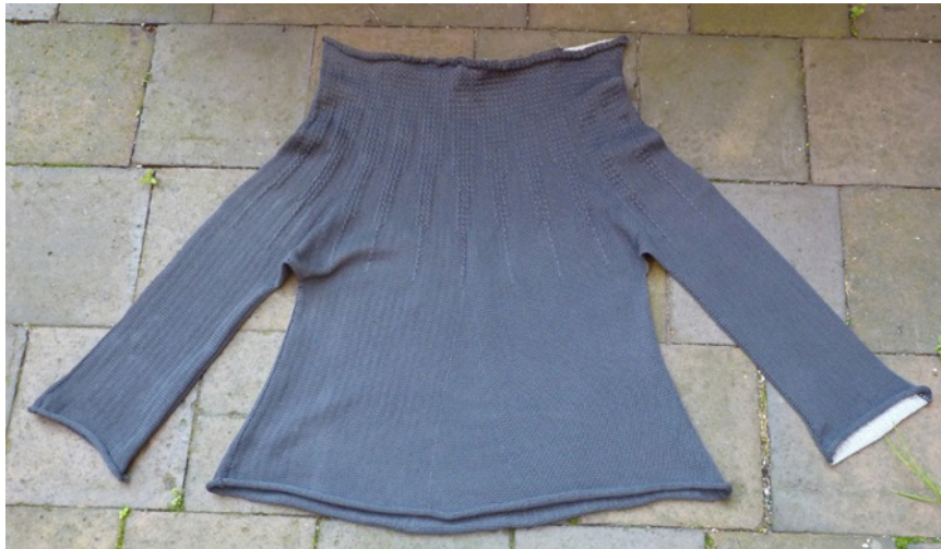
Figure 8.30. Sideways Seamless garment, produced on a Passap Duomatic hand-flat machine. (J.Taylor 2014)
