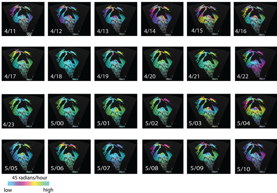
Fig. 11 24 interferograms of Soufrière Hills Volcano taken from the Montserrat Volcano Observatory site, created by averaging 1-min interferograms in hourly ( n ) stacks [ n:20 to (n + 1):20 ] on 4–5 August 2013. Image labels give the day/ (n + 1) hour in local time
