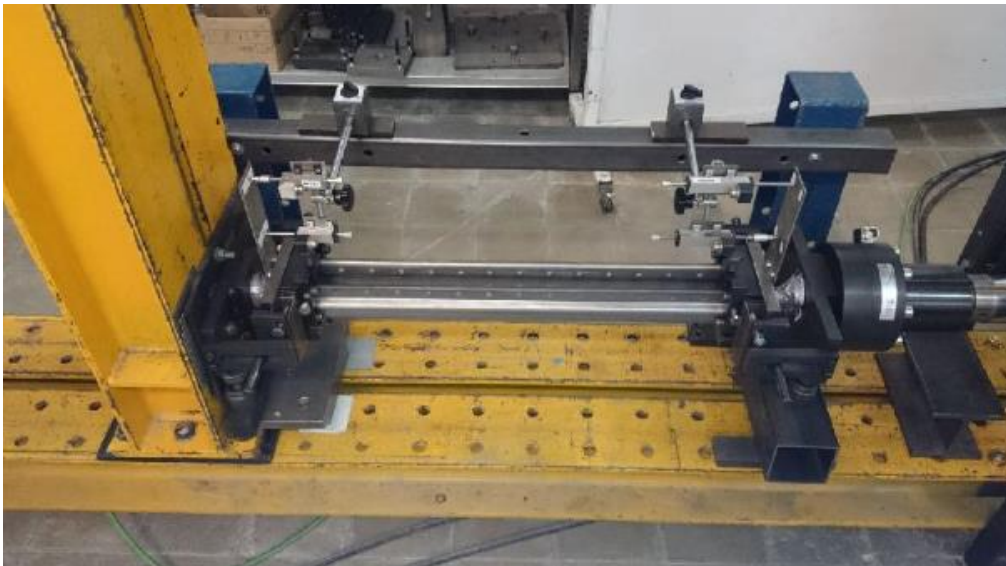
Figure 8: Set up of the displacement transducers used to obtain the axial displacement of the rack upright
