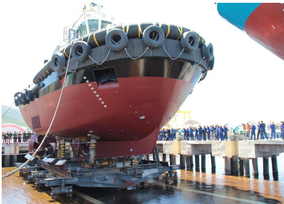
Figura 38. Sincrolift - [www.motorship.com](http://www.motorship.com)
