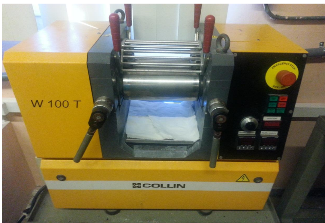
Open two-roll mixing mill
