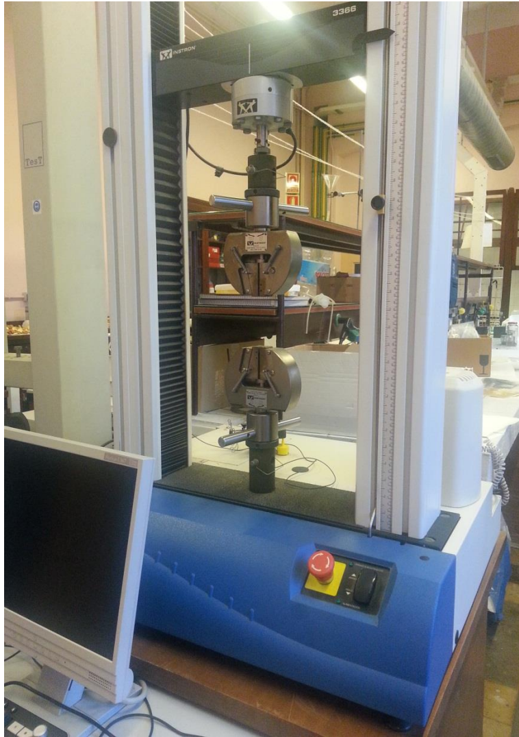
Bluehill Instron 5569 tensile machine
