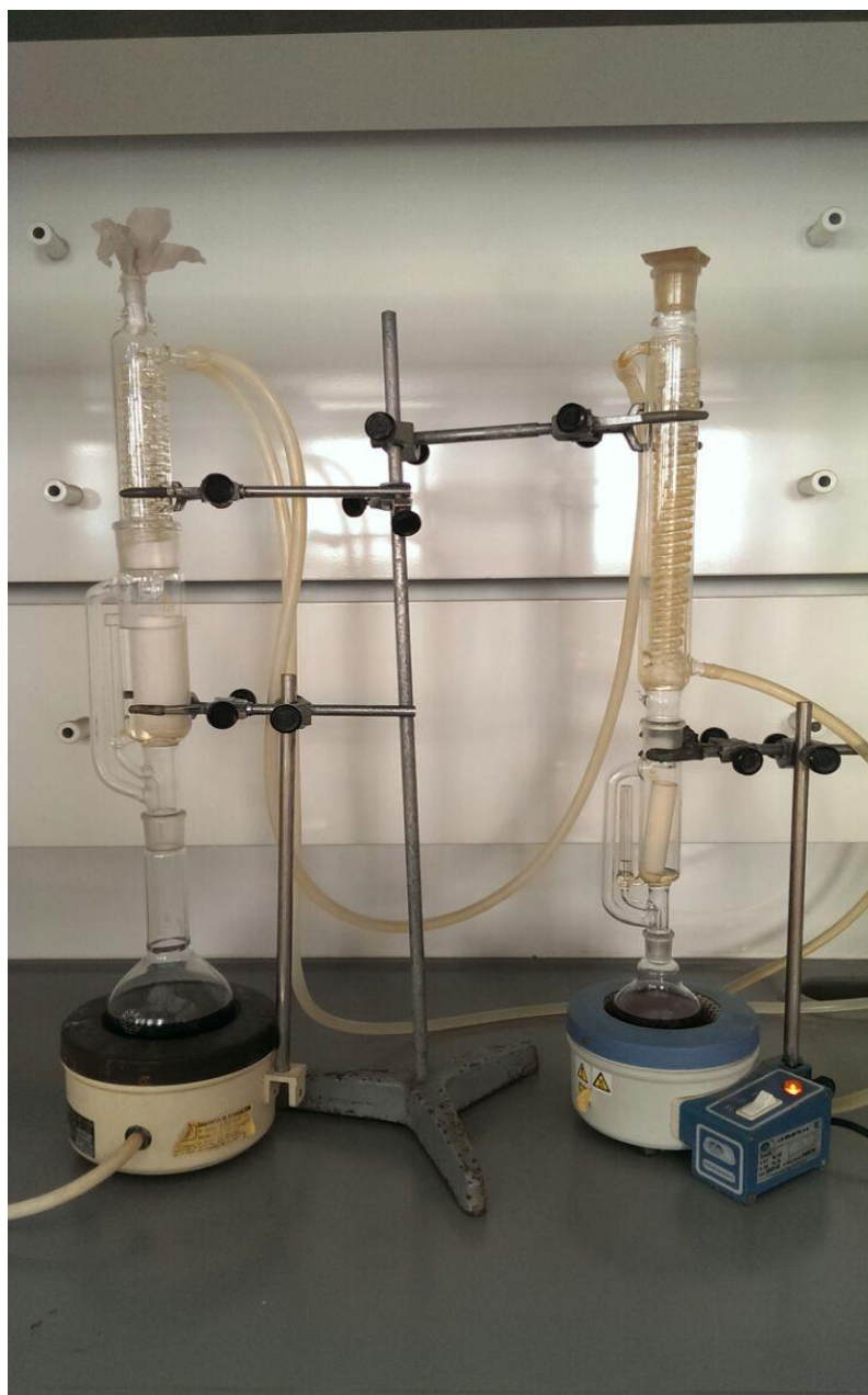
Soxhlet extraction apparatus
