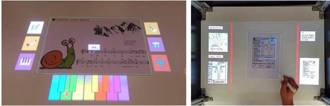
Fig. 1: Applications of our HDI system for (left) interpreting and interacting with a musical score in a public library and (right) automating a business work-flow (laboratory simulation).
