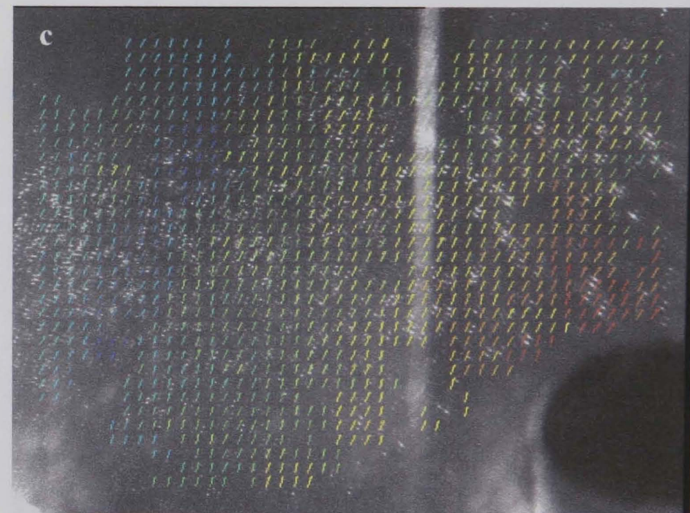
Figure 7.2. Example of the data set recorded between the ngvs. Colour bar is in \text{ms}^{-1} , Coordinates are in mm. Processed using autocorrelation (64 x 64 pixels).
