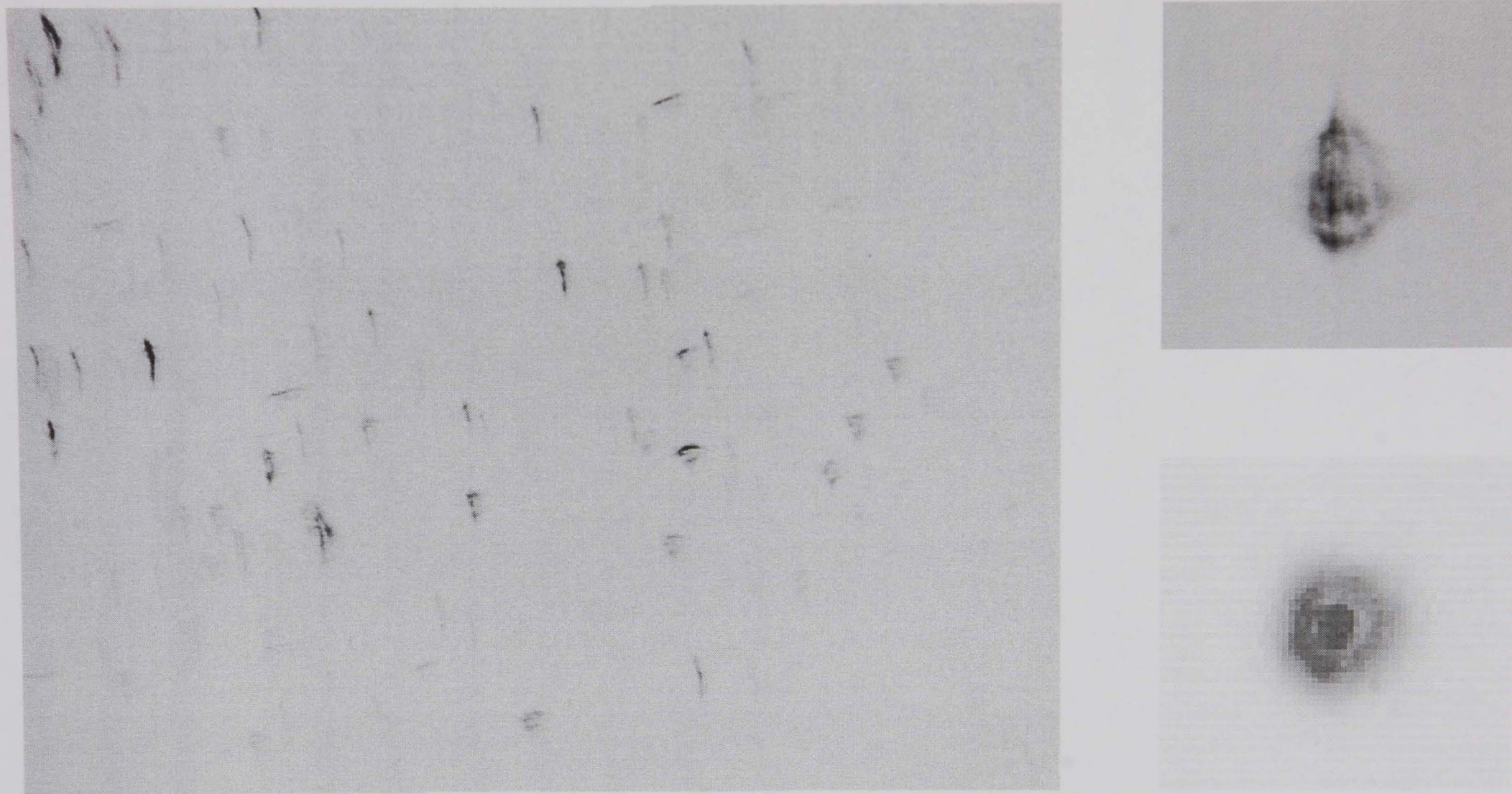
Figure 5.12 a. Diffraction image recorded through test-section window of turbine cascade (inverted). b. Single diffraction image recorded through window after partial correction with cylindrical lenses (inverted). c. Diffraction image taken from calibration for comparison (inverted).
