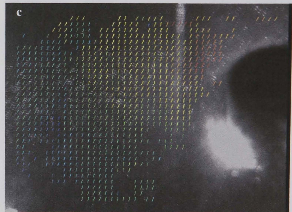
Figure 7.3. Example of the data set recorded between the ngvs. Colour bar is in \text{ms}^{-1} , Coordinates are in mm. Processed using autocorrelation (64 x 64 pixels).
