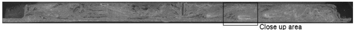
Figure 11.1 - A cold rib tool GMT moulding at 60 bar over 1 second, with oven temperature of 200°C
