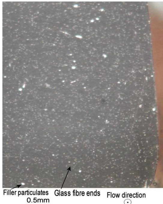
Figure 11.10 - Micrograph showing glass orientation at end of top flange of section 5, small white dots denote glass fibre ends, larger white dots denote filler particulates. The flow path is towards the reader.
