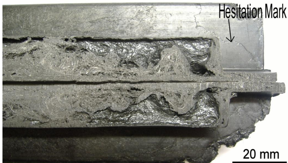
Figure 10.3 – Photo showing rib tool GMT moulded with parameters 60 bar, 50°C tool temperature and 200°C oven temperature. It contains a smooth cavity and hesitation mark
