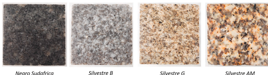
Fig. 1. Photograph of the four types of granites used in the experiment (from low to high bioreceptivity index).
