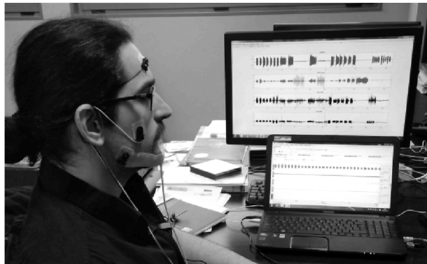
Fig. 3. Recording the myoelectric surface signal produced by the contraction of the masseter and the 2D acceleration in the sagittal plane.
