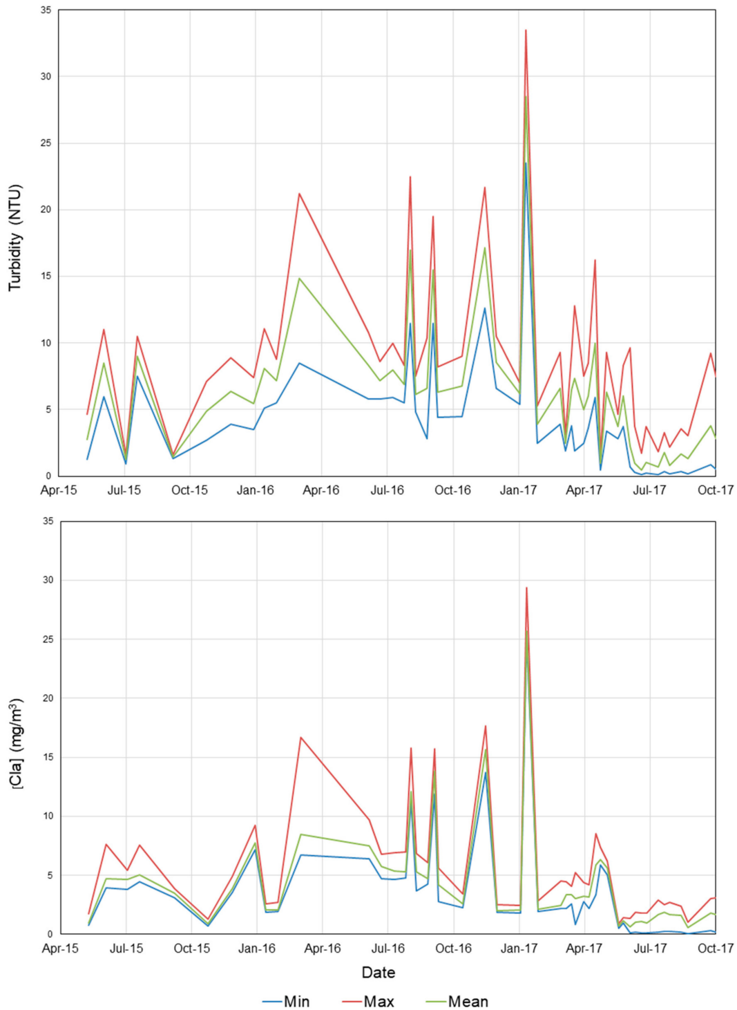
Figure 6. Time series of the maximum, minimum, and mean values of water parameters, estimated from satellite images.
