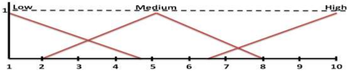
Fig. 5.3-9 Thermal variation membership function (DLC criterion)
