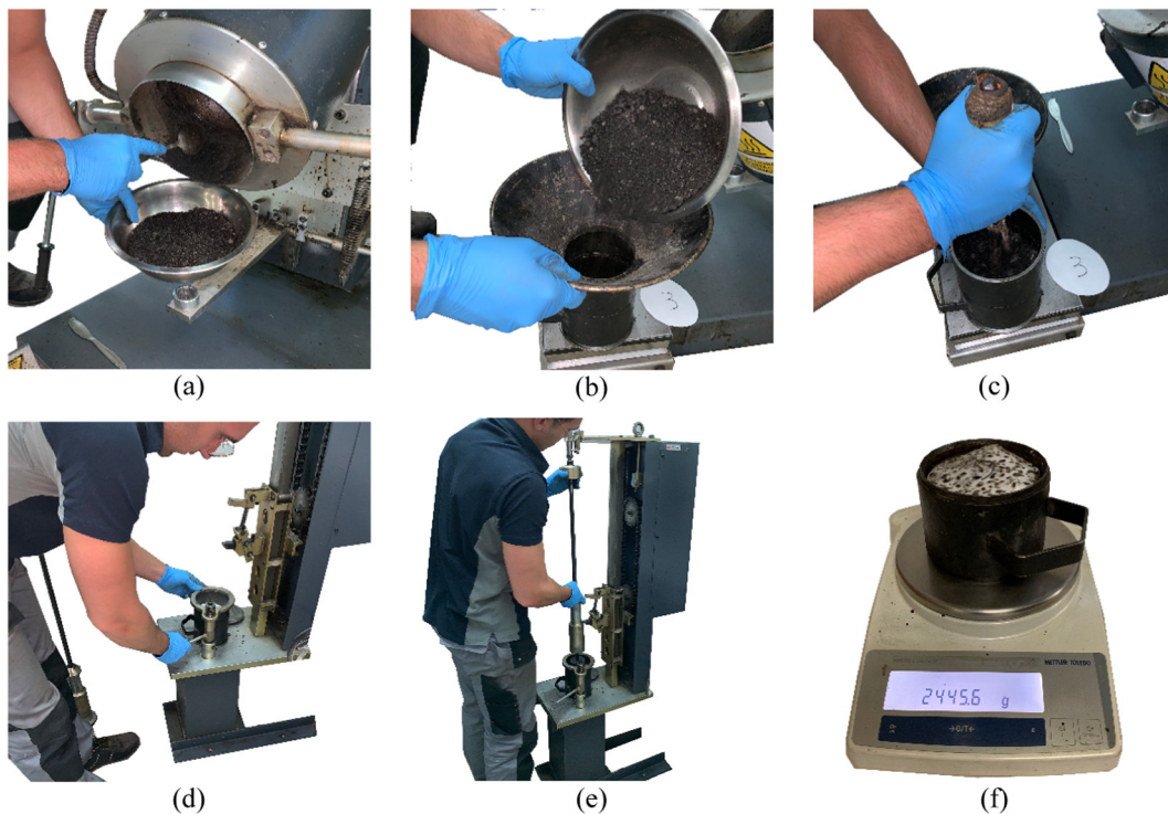
Fig. 5. Impact compaction procedure: (a) Sample mixing; (b) Sample placement; (c) Sample placement II; (d) Mould placement; (e) Hammer placement; (f) Compacted specimen weighing.
