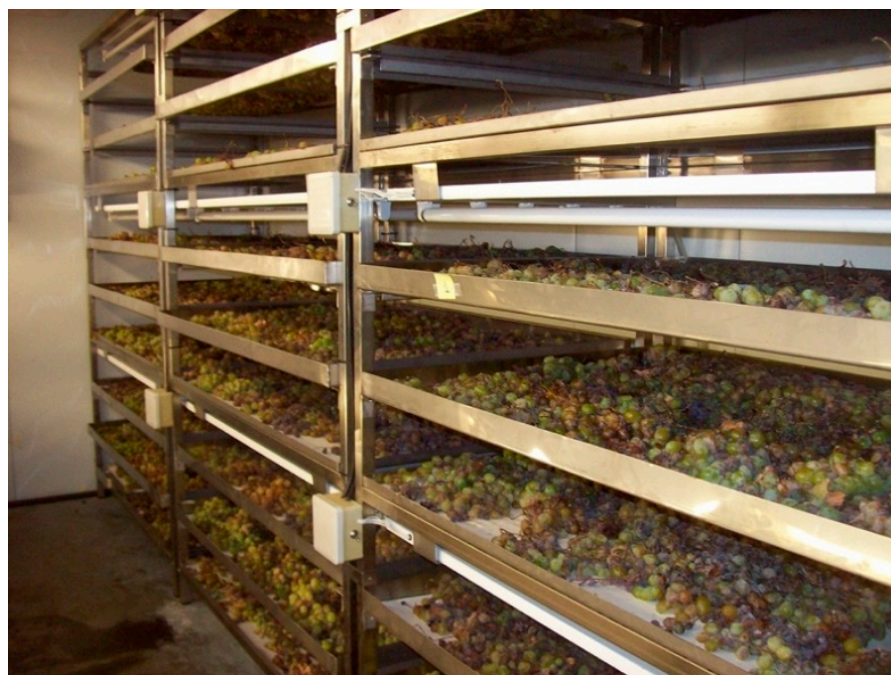
Figure 4. Climatic chamber with temperature and moisture control.
