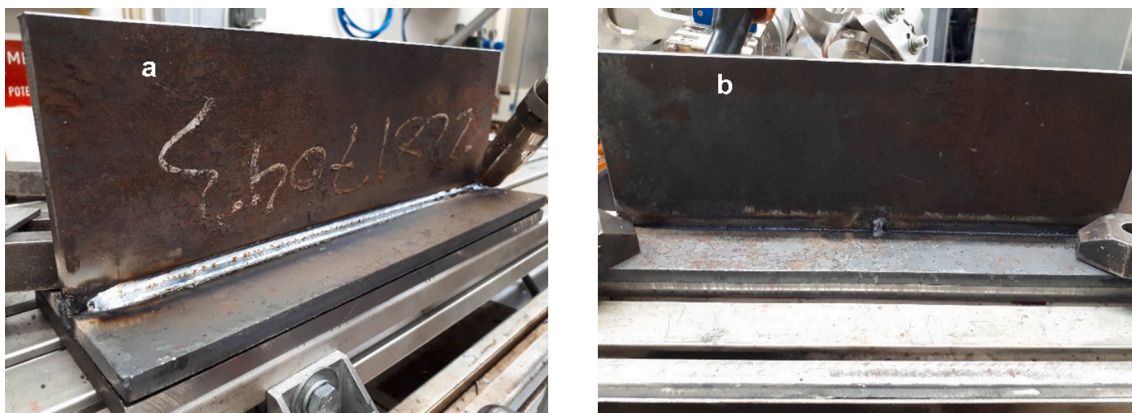
Fig. 7. Image of weld seam of a HLAW T weld. a) Face side; b) Root side.
