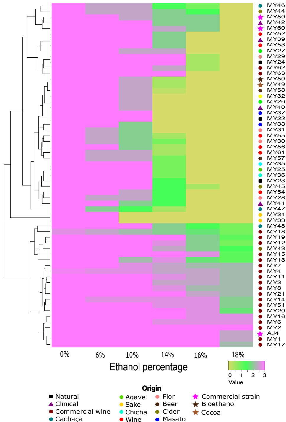
FIGURE 1.2 Heatmap representation of growth values (from 0 to 3) of the analyzed strains at plates with increasing ethanol concentrations. Each line corresponds to a strain (AJ4, MY1-MY63) and each column to a particular ethanol concentration (0%, 6%, 10%, 14%, 16% and 18%). The color key bar at the top indicates growth values, from yellow (low growth value) to pink (high growth value). Hierarchical clustering is showed on the left. Color dots on the right of the Figure indicate the source/origin of each one of the strains. In Supplementary Figure 1 can be seen one of the four replicates from which these heatmap was constructed.
