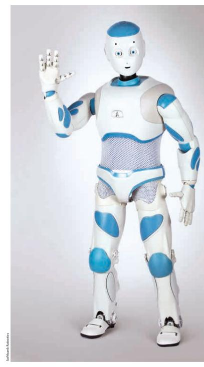
One of the criticisms of non-corporeal artificial intelligences is that an intelligent agent needs a body to be able to experience the world directly. The picture shows the Romeo humanoid robot developed by SoftBank Robotics.
