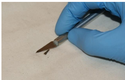
Fig. 6. Example of a small wood fragment collected for identification
