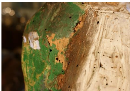
Fig. 2. An artwork deeply attacked by xylophagous insects as seen by the numerous holes
