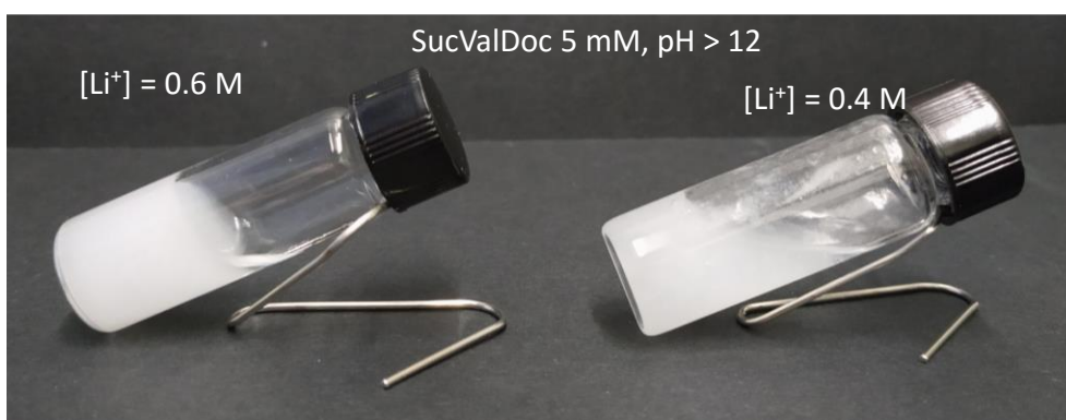
Figure 3.16 Picture of vials showing the influence of alkaline cation concentration on gel formation.
