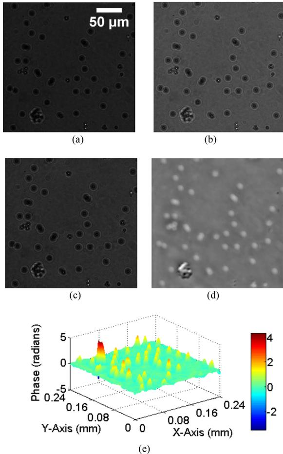
Fig. 4. Experimental results of multi-plane phase imaging. (a)–(c) Three out of focus images of microbeads, (d) the 2D phase distribution obtained from images (a)–(c) by using the TIE algorithm, and (e) quantitative phase profile. The intensity image shown in Fig. (b) and the phase image shown in Fig. (d) are used for further processing to retrieve other focused phase images.
