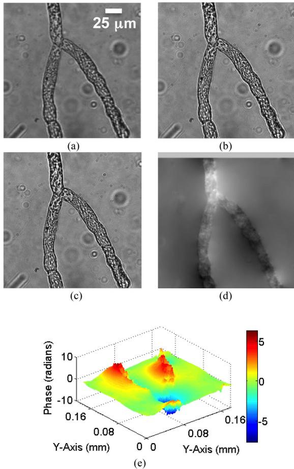
Fig. 6. Experimental results of multi-plane phase imaging of plant cells. (a)–(c) Three out of focus images of living plant cells, (d) 2D phase distribution reconstructed from defocused images by using the TIE algorithm, (e) 3D plot of the phase distribution.
