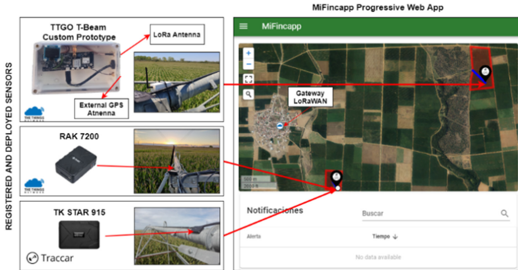
Fig. 6 – Sensors deployed on the MiFincapp platform in the maize fields of Pobladura de Pelayo García, León, Spain.
