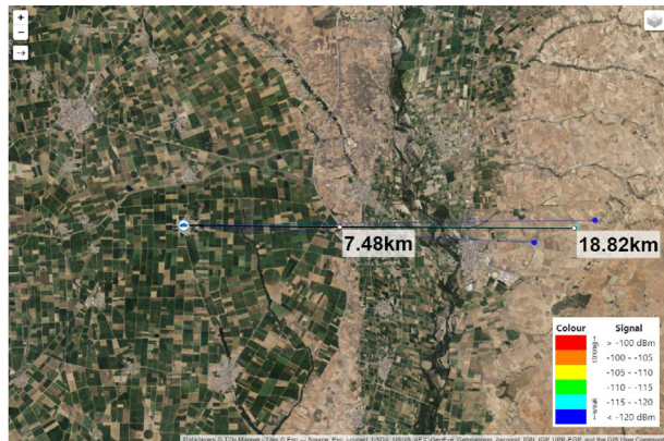
Fig. 8 – LoRaWAN test coverage at near crops.
