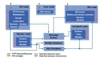
Fig. 3. Cloud microservices architecture.
