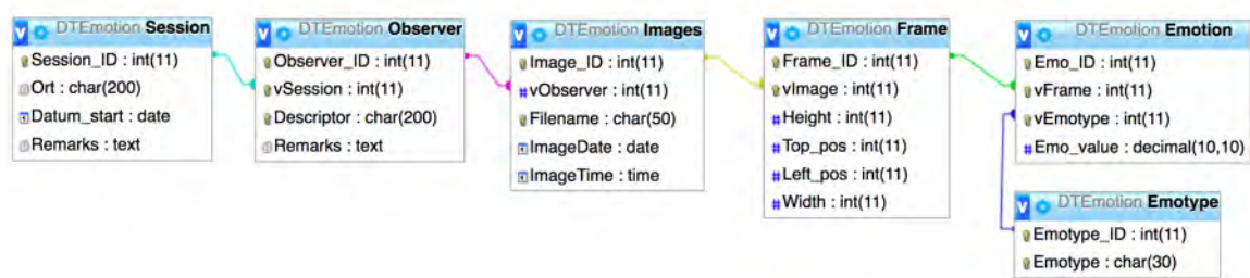
Figure 57. Project One – Database Structure for the Data Gathering of the Emotion Recognition Project – Devised by author
