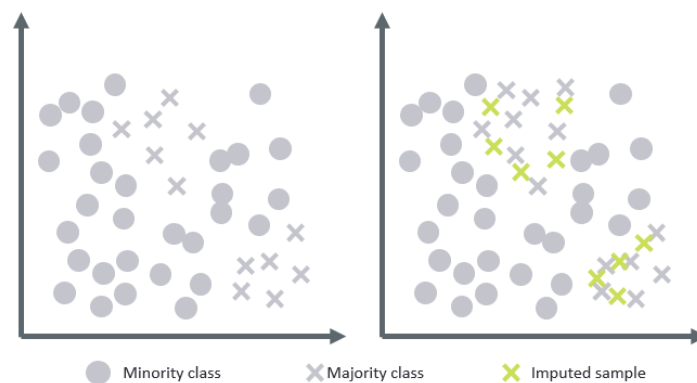
Figure 2 - A two dimensional schema of the Borderline-SMOTE algorithm. The imputed samples are imputed between the points closest to the boundary between minority and majority class.
