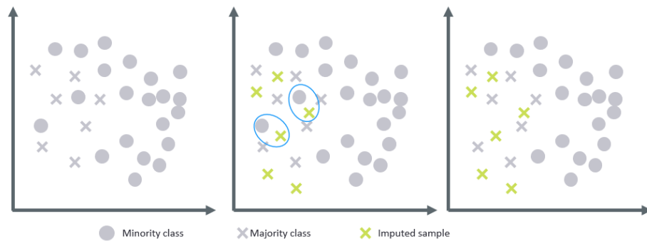
Figure 3 - A two dimensional schema of SMOTE-Tomek. Majority samples within the space of the minority samples are filtered out after samples are imputed in this space.
