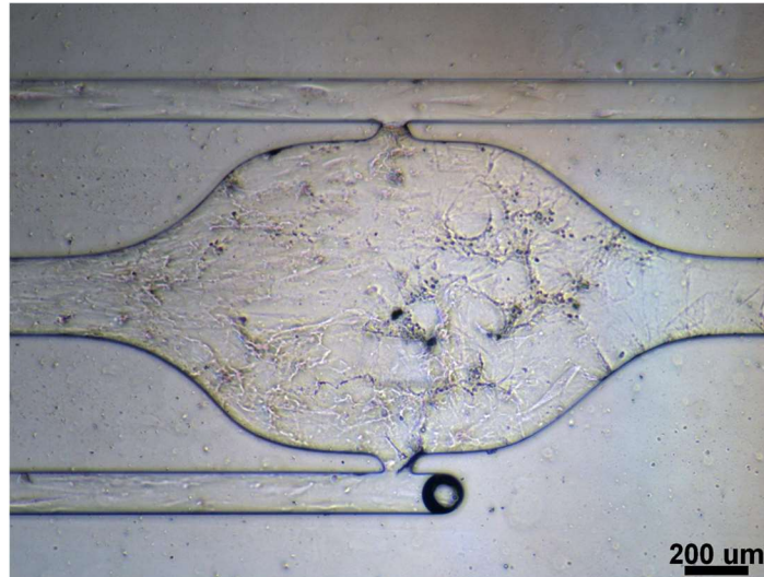
Figure 3.13: Chip on which after immunofluorescence was made trypsinization. Cell debris remains inside the chambers, making it impossible to reuse.
