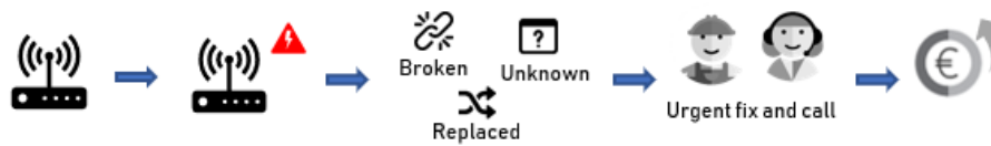
Figure 1.1: A RM example: STB running for an unknown reason and the client has to call to the technical support, this unplanned intervention is more expensive than scheduled one for the company.
