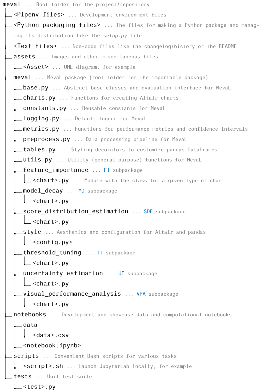
Figure 3.1: Approximate project structure for Meval. The __init__.py files for the package and each subpackage are omitted. The preprocess.py file contains all the functions to preprocess raw datasets and create datasets (pandas DataFrames) ready to be plotted.
