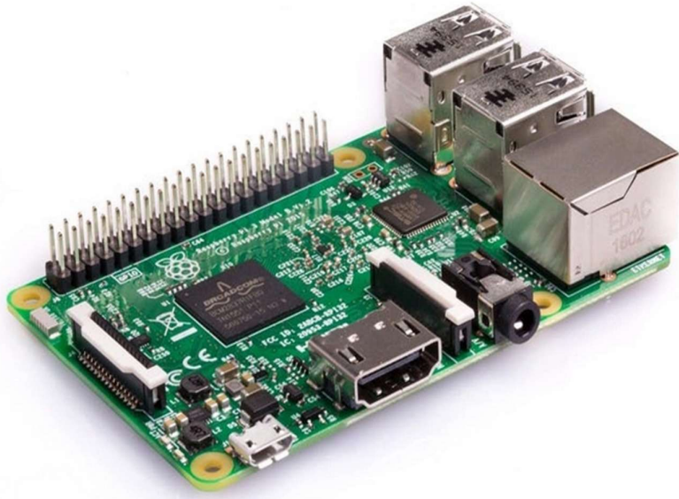
Figure 7: design of a raspberry Pi 3 Model B Single Board Computer
