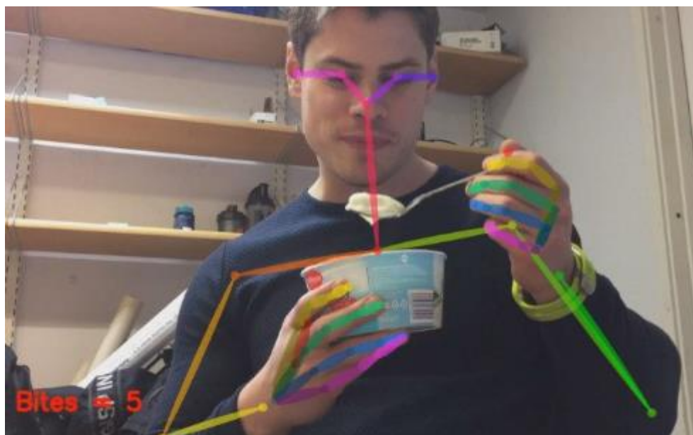
Figure 22. Visual illustration of skeletal extraction for algorithm estimations of number of spoonfuls during a meal by an early version of the bite/spoonful counting algorithm "Rapid Automatic Bite Detection".
