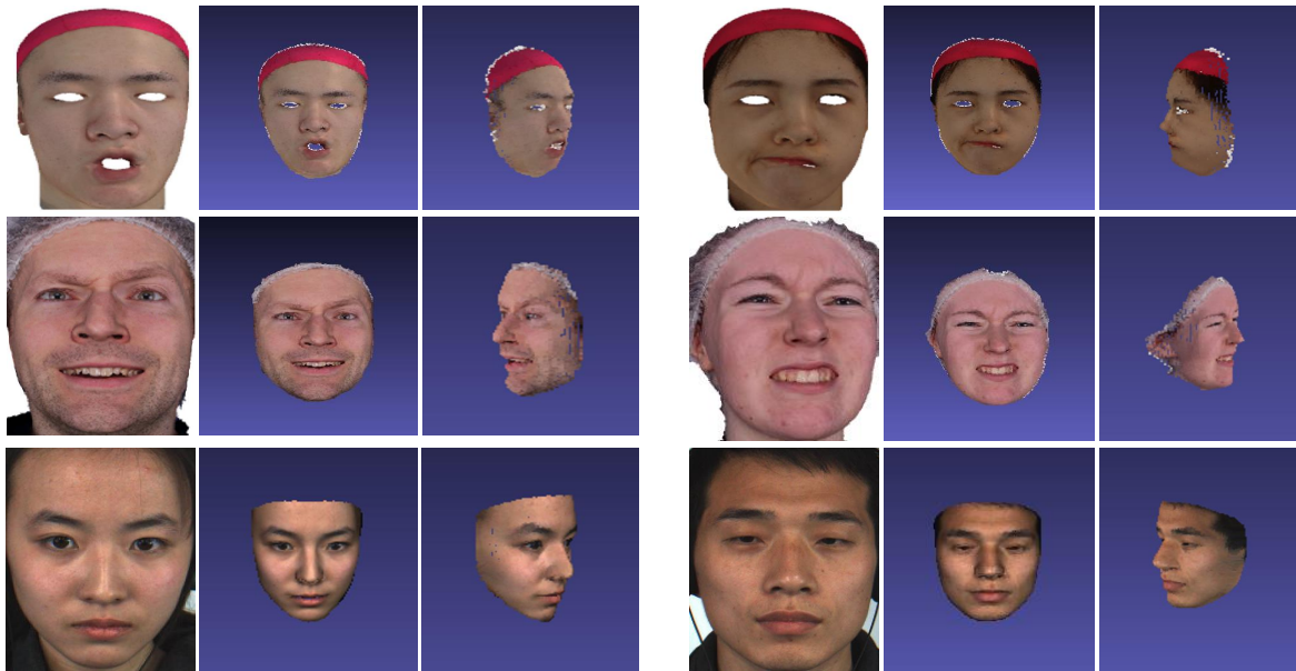
Fig. 7. Given a single color face image of frontal view, our method can produce a high-quality mesh (depicted in two different perspectives) that contains correct global shape and detailed textures on organs. Top to bottom: Examples from test split of Facescape dataset; Examples from test split of Stirling ESRC 3D face dataset; Examples from facial micro-expression CAS(ME) 2 dataset;
