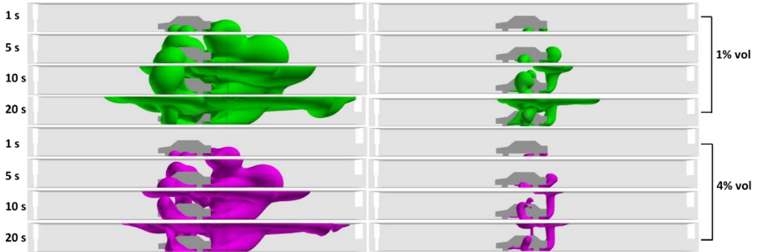
Figure 15. Side view of iso-surface plots for 1% and 4% vol of hydrogen mole fraction for case 4 (2 mm TPRD, left) and case 9 (0.5 mm TPRD, right) with 0° angle downward release and tank blowdown.
