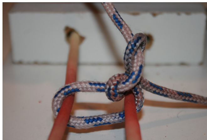
Figure 13 Final effect of pulling on one end of reef knot leading to loosening of knot.
