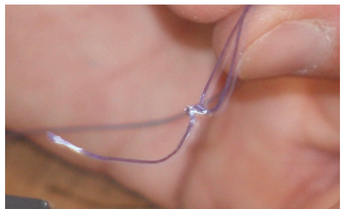
Figure 7 Minimal slippage of knot prior to rupture of loop in suture by distraction in test bed.
