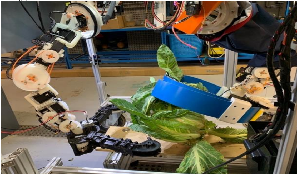
Figure 10: cutting robot arm & picking robot arm
