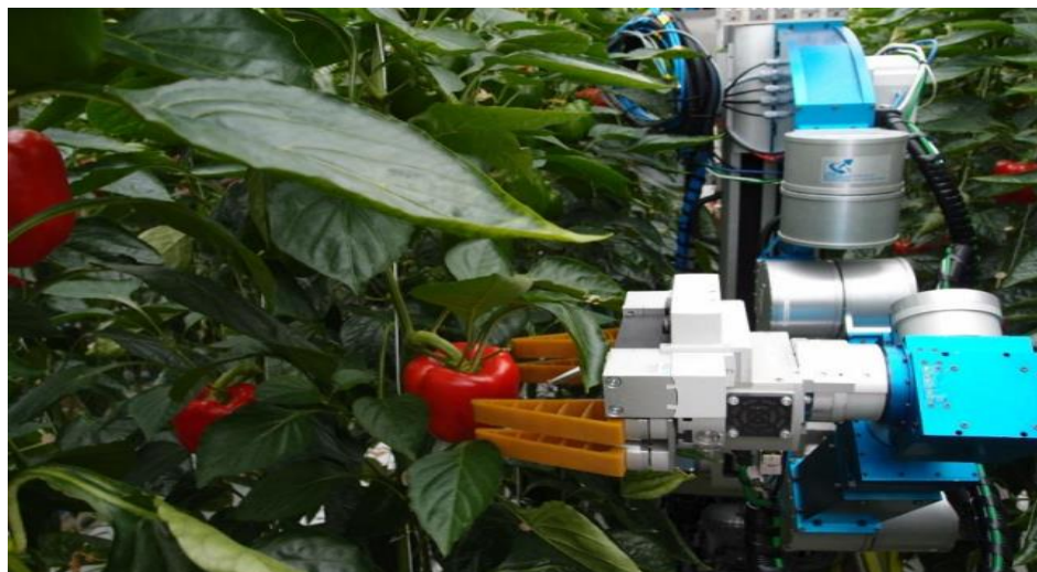
Figure 2: tomato Harvesting robot inside greenhouses.
