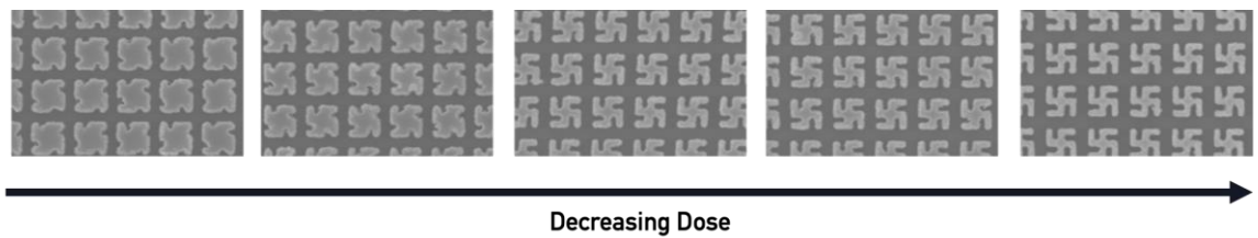
Figure 3.7: The effect of electron beam dose on gammadion morphology
