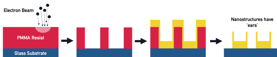
Figure 3.4: Using only a monolayer of resist results in 'ears' on the finished structure.
