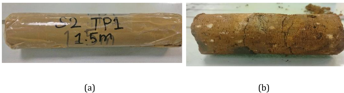
Figure 4.7 (a) Sample core obtained from the field, (b) sample extruded from the core.
