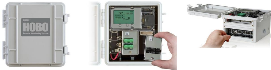
Figure 5.8 HOBO RX3000 remote monitoring station data logger. Source: ONSET (2019, n. Date accessed: 16-06-2020).
