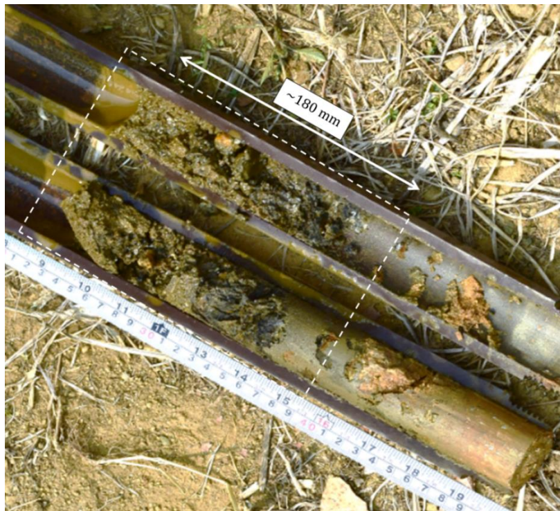
Figure 3.6 180 mm thick weathered cobble extracted by the SPT sampler in BH-1 at 3 m.
