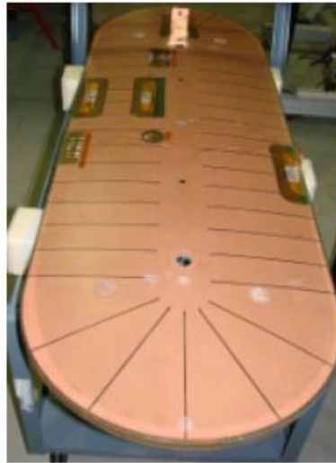
Figure 3.8. 2G HTS pole set designed and tested for a 10 MW class generator [18].
