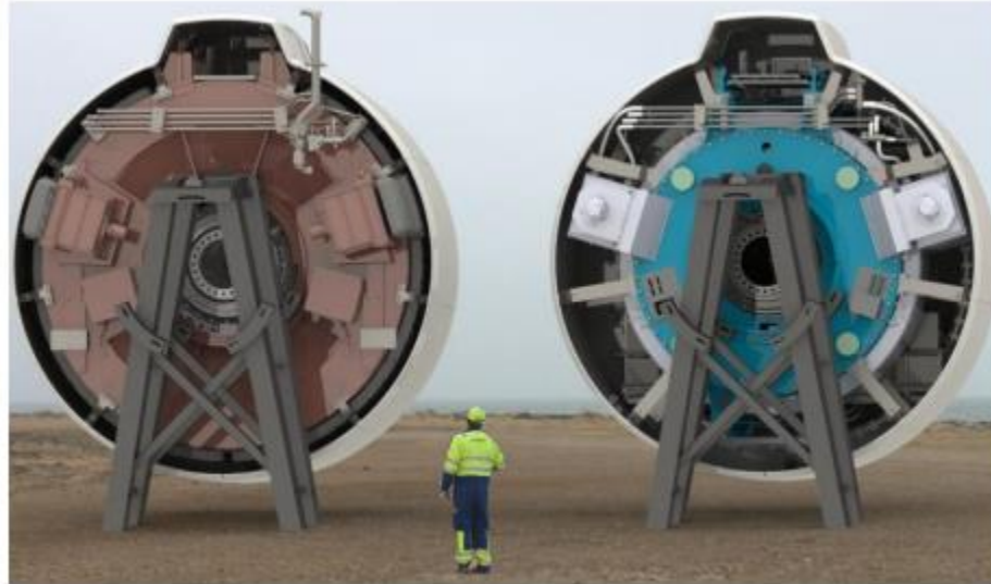
Figure 1.5. PM generator (left) and EcoSwing generator (right) [20].
