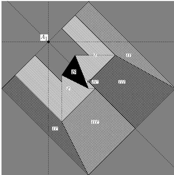
Figure 3.3: The complete partition of a large \mathcal{P} with one existing facility A_1 = (0, 0) and a barrier \mathcal{B} with vertices (2, -5) , (4, -2) , and (6, -7) .
