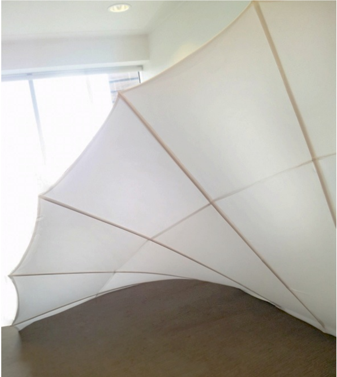
Figure 5-14: The Double Twist space divider actual model, scale 1:1, and the ‘Boned Draping’ method, which employ textiles’ malleability to achieve stability and express interdisciplinary understanding.
