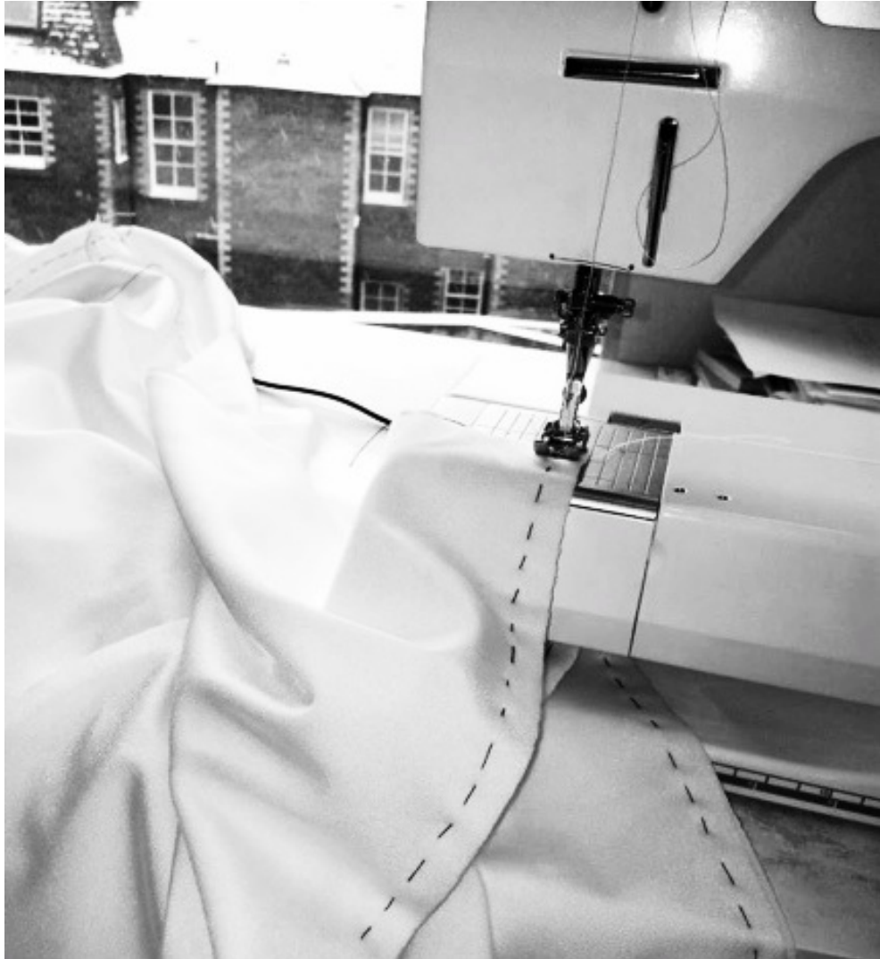
Figure 4-42: Hand stitching was conducted prior to machine stitching to keep the edges of patterns together and prevent slippage.
