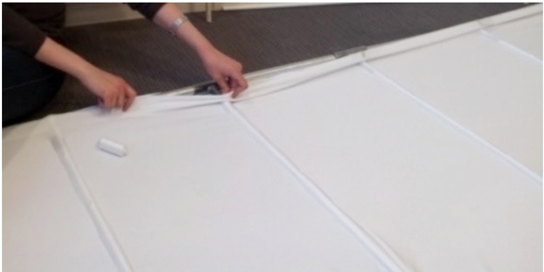
Figure 4-47: Installation process. Left and middle: inserting ribbing into the sewn fabric channels. Right: finishing the waistband detail to cover the bottom rib, using hand stitching.
