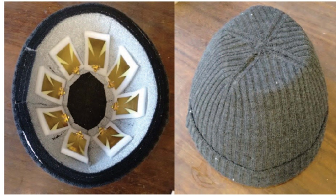
Figure 2.13: First prototype of wearable microwave head imaging device with thin flexible antennas on PET-film substrate [132].
