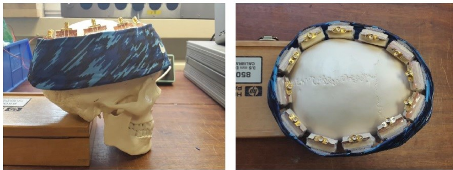
Figure 2.14: Wearable head strap-based microwave imaging device with textile-based antennas [132].
