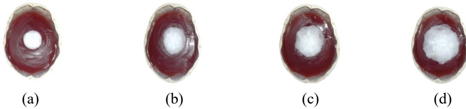
Figure 5.11: Fabricated phantoms with the following volumes of the AD-affected brain tissues: (a) 22.6 \text{ mm}^3 , (b) 56.5 \text{ mm}^3 , (c) 113 \text{ mm}^3 , and 226 \text{ mm}^3 .
