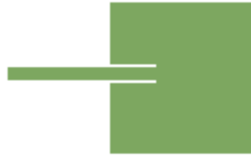
Figure 3.11: Antenna with inset feed line.
