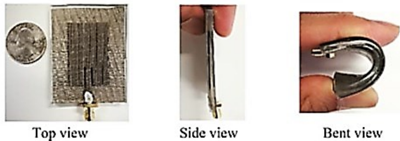
Figure 3.5: Images of the fabricated PDMS-embedded conductive fabric antenna [168].
