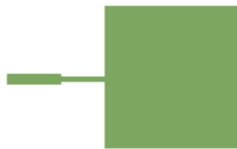
Figure 3.12: Antenna with quarter wavelength transmission line.
