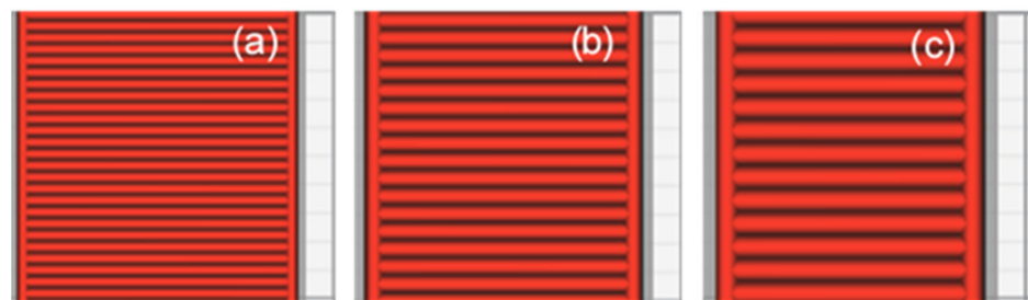
Figure 3. Nozzle size: (a) 0.4 mm; (b) 0.6 mm; (c) 0.8 mm.
