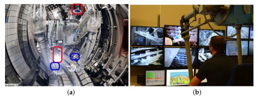
**Figure 2.** JET's remote handling system: (a) MASCOT manipulator (robotic system) inside the JET vacuum vessel; and (b) operator, interface and viewing system. Red and blue squares represent the HD and ancillary cameras, respectively, mounted on MASCOT.
