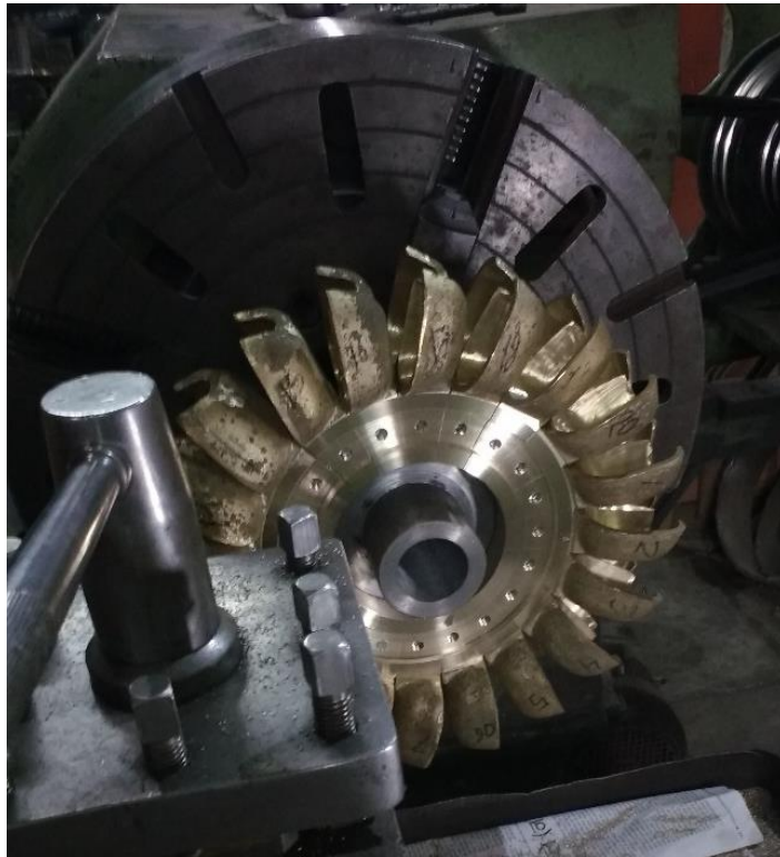
Figure 6.6 - Machining operation on a Pelton turbine runner. Photo credit, author.
