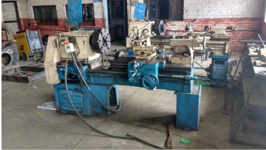
Figure 6.11 – An engine lathe in a workshop. Photo credit: author.
