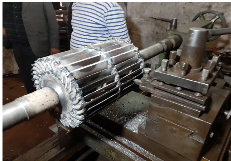
Figure 6.8 - Machining operation on a Crossflow turbine runner. Photo credit, Topaz Maitland.
