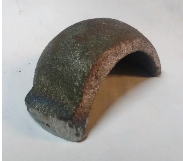
Figure 6.42 - Cast steel blade before machining. Photo credit, author.
