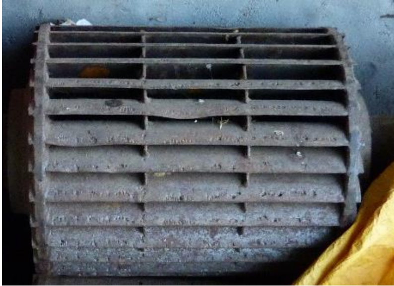
Figure 4.6 - Abrasion on a Crossflow turbine runner. Photo credit, author.
