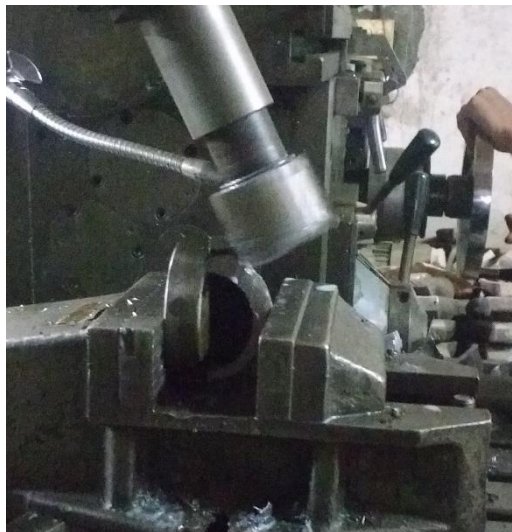
Figure 6.43 - Machining process on the steel blade. Photo credit, author.
