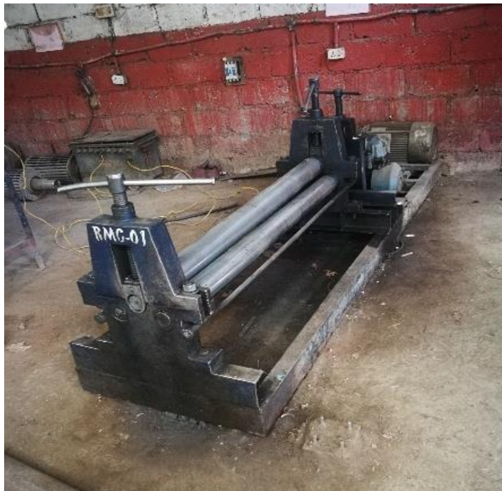
Figure 6.12 - Roller bending machine in a workshop. Photo credit: Topaz Maitland.
