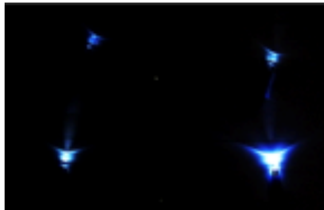
Figure 3.11 The simulated circuits for each of the fibres (top) and the brightness of LED (bottom). Clockwise from top left the fibres are: PEDOT:PSS-ALG, PEDOT:PSS-ALG (150 °C), PEDOT:PSS-ALG-PEG (150 °C) and PEDOT:PSS-ALG-PEG in the bottom left.
