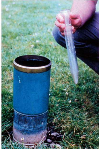
Figure 2-1 'Snowdon' rain gauge and graduated cylinder (Strangeways, 2010).
