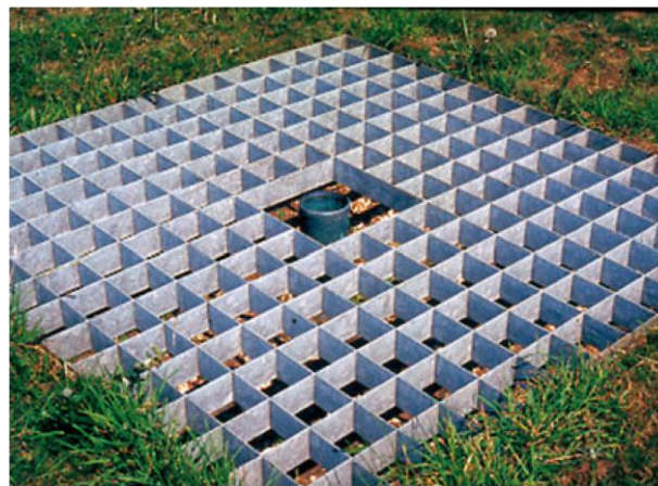
Figure 2-3 Pit rain gauge (Strangeways, 2010).
