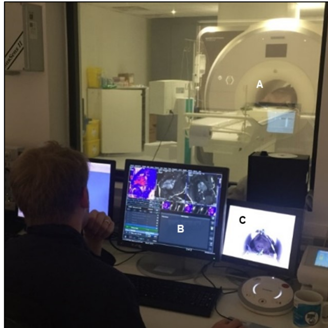
Figure 18. TBRC MRI suite seen from the control room. Animal under anaesthesia positioned in the scanner (A and C); cardiac image acquisition ongoing (B)
