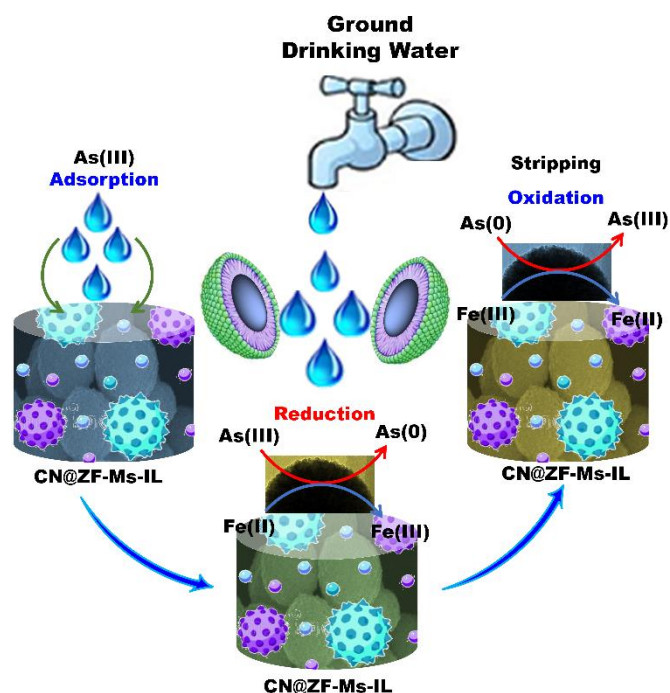
Scheme 2 Schematic diagram showing sensing mechanism of our designed sensor towards As(III).
